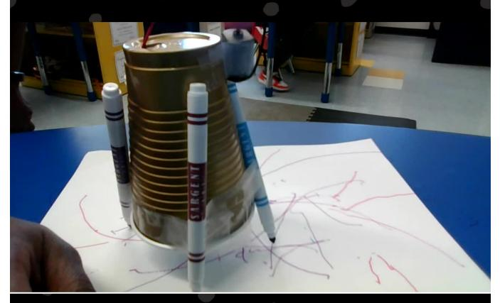
This is a Scribble Bot that we made. Scribble Bots are also easy to create. Our Scribble bot is made out of a cup and it has 4 markers for legs and a motor with wires and a battery pack.
